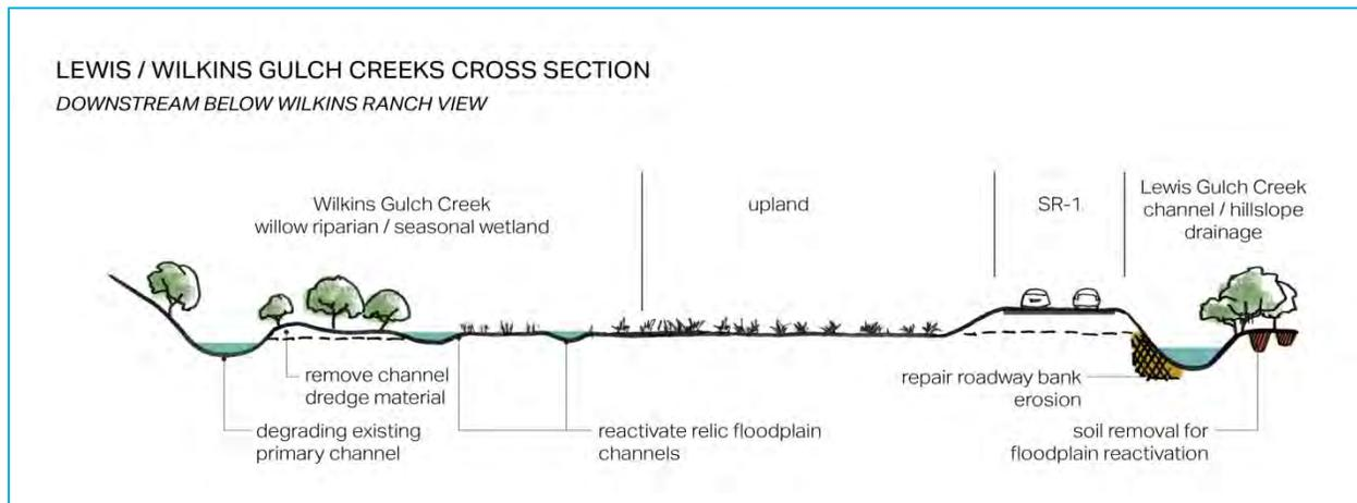
The geometry of the meander bend and streambank may require minor grading of the creek bed to provide adequate space to rebuild the eroding bank (see Figure 18) and maintain channel capacity. The feasibility of a combined bioengineered and traditional engineered approach should be evaluated in more detail in a subsequent design stage.
